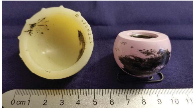
Figure 2: The acetabular liner (left) with deep and shallow scoring, with the longest on the lower right with a length of approximately 2.0cm. The ceramic head (right) showing broad amounts of wear as well.
