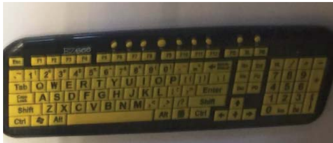
Figure 4. Reflected image of a high contrast keyboard with large letters. All the letters are visible and easily recognizable in the reflected image. The room light source is located on the left side of the keyboard; this is why the left side of keyboard looks brighter than the right.
