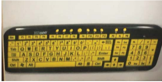
Figure 2. A reflected image of the keyboard with high contrasting letters color and large letters.
