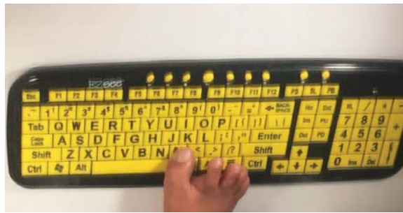
Figure 3. Toe pressing letter 'M'. The figure presents the use of toe. The image is a reflected one that appears in front of the user. The keyboard was lit by the LEDs.
