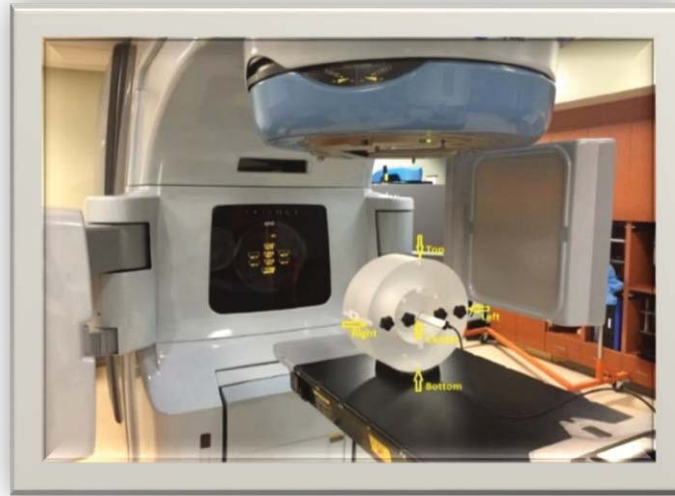
Figure 1: Imaging dose measurement set up using Unfors Xi and CTDI phantom
